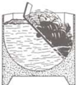
2. Birds are dumped to bottom of tank—water sprays through holes in platform on to birds.
